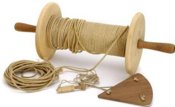
out. Knots placed at a distance of 47 feet 3 inches (14.4018 m) from each other, passed through a sailor's fingers, while another sailor used a 30-second sand-glass (28-second sand-glass is the currently accepted timing) to time the operation. The knot count would be reported and used in the sailing master's dead reckoning and navigation. This method gives a value for the knot of 20.25 in/s, or 1.85166 km/h. The difference from the modern definition is less than 0.02%.
